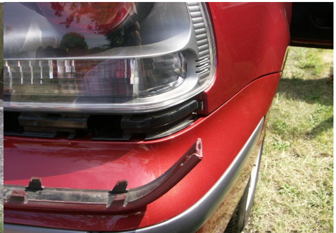
Picture 3. Locate the leading edge first when refitting.
