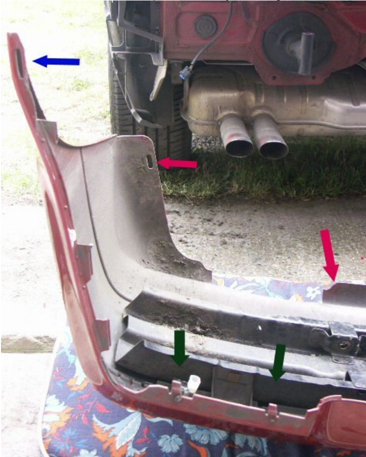
Picture 2. The trim clips out easily.
