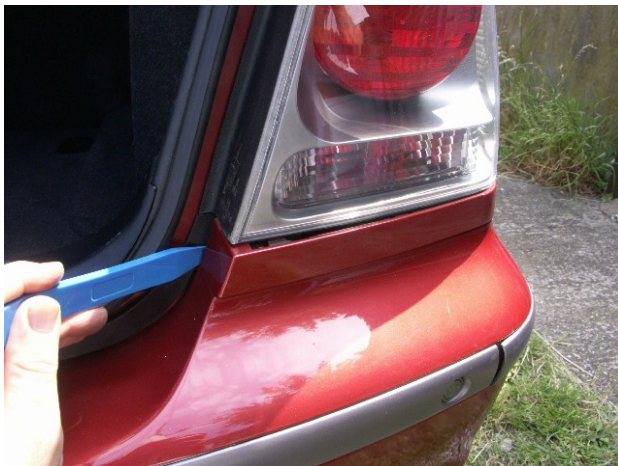
Picture 2. The trim clips out easily.
